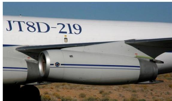
**Pratt & Whitney JT8D-219 engine on the 707RE flight test aircraft (Alan Radecki 2007)**
