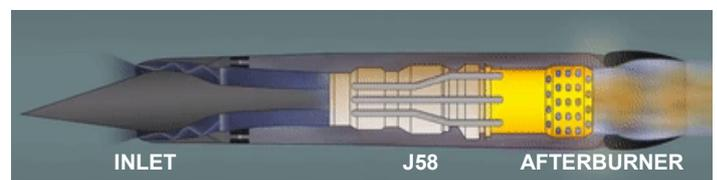
**Figure 7 Basic composition of the SR-71 engine nacelle**
