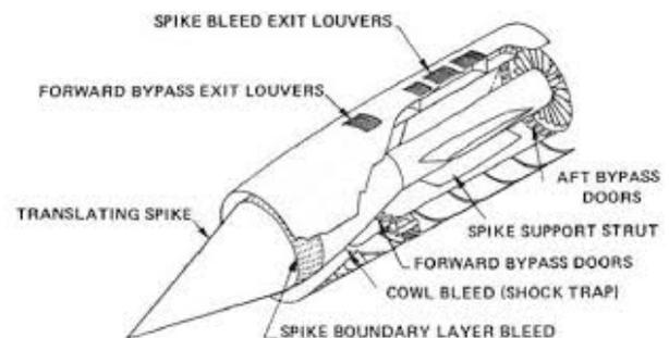
**Figure 12 Key parts of the forward section of the nacelle**
