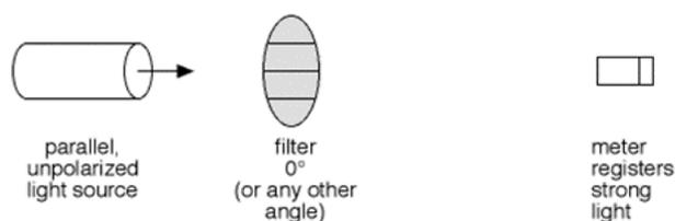
Figure 2 - a one-filter setup
