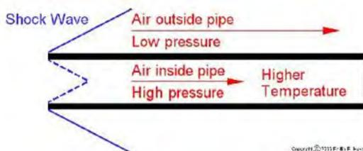
**Figure 6 A hollow tube experiencing supersonic airflow**
