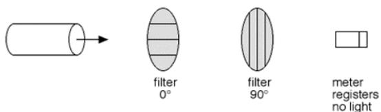
Figure 3 - a two-filter setup
