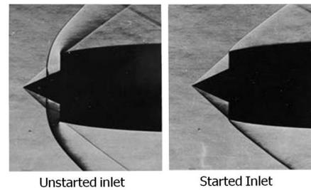
**Figure 11 Shockwaves at a started inlet vs an unstarted inlet**
