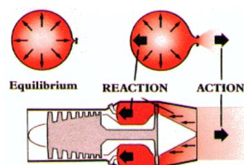
Figure 1 Action reaction force pairs in a balloon and a jet engine
