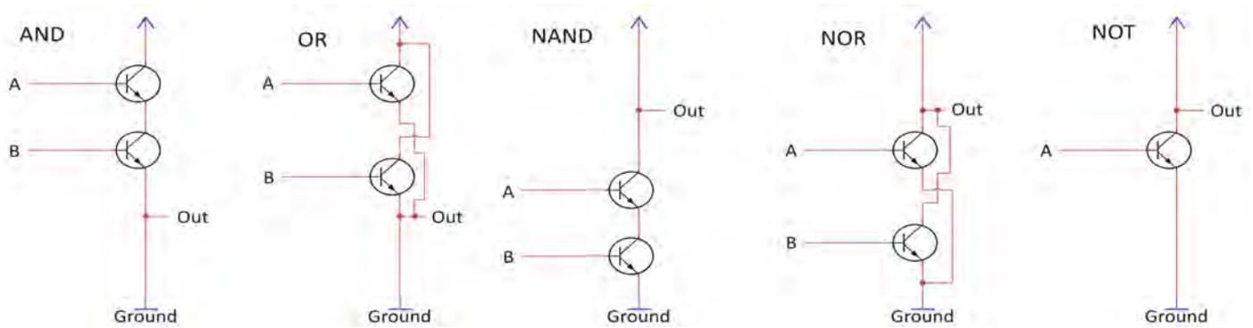
Figure 1 - Transistors used to make logic gates
