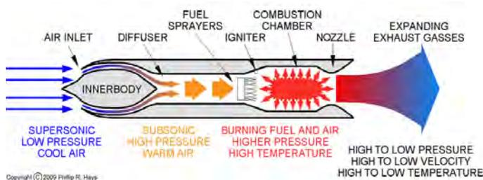
Figure 3 A ramjet engine
