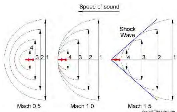
Figure 5 Pressure waves around aircraft at various speeds
