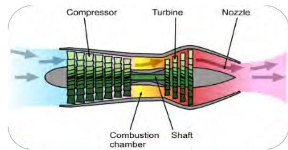
**Figure 2 A turbojet engine**
