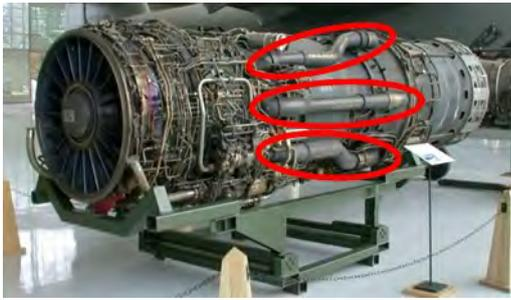
**Figure 8 Bypass tubes on a J58**
