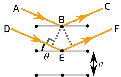
**Fig. 1: X-rays interacting with a crystal. See if you can try deriving Bragg’s law, the conditions required for constructive interference, in terms of  $\theta$ , the atomic spacing  $a$ , and the wave-**
