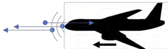
Figure 4 Air molecules interacting with a subsonic aircraft and pressure waves formed
