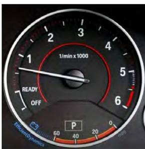
**Tachometer on a BMW, with redline between 5500 RPM and 6000 RPM**
