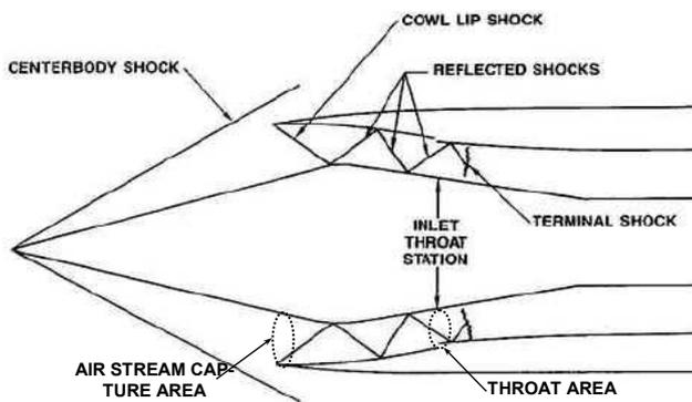
**Figure 10 Shockwaves formed in the inlet**
